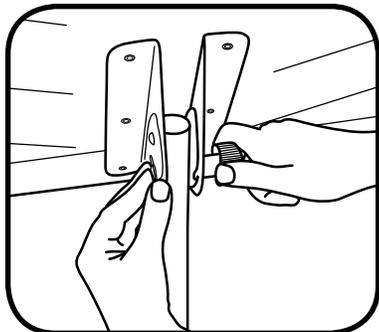
**CAUTION:** Avoid using any type of lubrication on height adjustment shaft, as this may cause the unit to slip.
