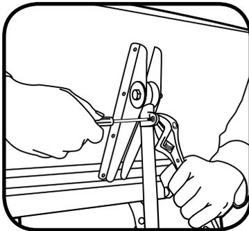
**CAUTION:** Avoid using any type of lubrication on height adjustment shaft, as this may cause the unit to slip.
